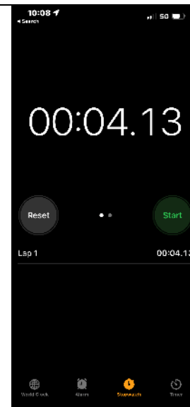
PHOTO #34: Door closing speed of 4.13 seconds at women's restroom on second floor (Non-Compliant)
