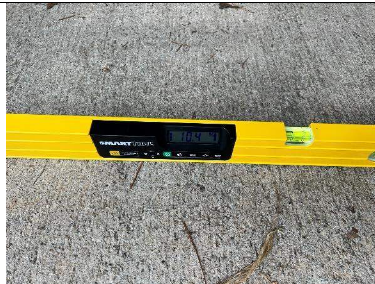
PHOTO #6: Running slope of 10.4% obtained (Non-Compliant). Running slopes on ramps should not exceed 8.3%.
