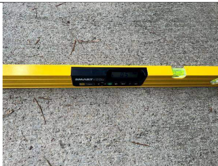
PHOTO #8: Cross slope of 0.5% obtained (Compliant). Cross slopes should not exceed 2.08%.
