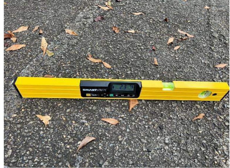
PHOTO #18: Running slope of 2.3% at access aisle (Non-Compliant). Running and cross slopes in access aisles and parking spaces should not exceed 2.08%.
