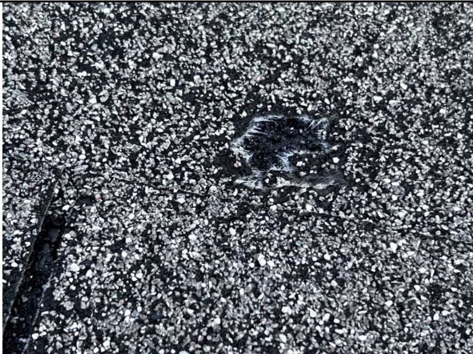
Photo 68: Hole in shingle, fiberglass reinforcing exposed
