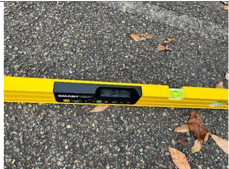
PHOTO #20: Cross slope measurement of 0.7% obtained (Compliant). Running and cross slopes in access aisles and parking spaces should not exceed 2.08%.
