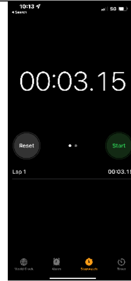
PHOTO #42: Door closing speed of 3.15 seconds at men's restroom on second floor (Non-Compliant).
